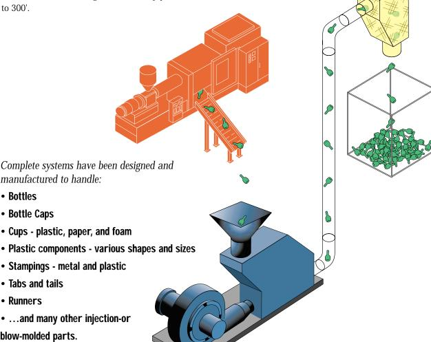
Sterling also provides similar systems designed to convey pellets or scrap parts where part integrity is not required. Systems can be custom designed to fit your particular application, including multiple pick-up points and various configurations.
