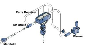
This system shows finished parts being collected from molding machines and delivered to their destination through tubing to a Parts Receiver. The use of a 2-Way Manifold affords the system the capability to pick up parts simultaneously from two different machines. The Air Brake slows down the parts before they enter the Parts Receiver, thereby minimizing impact and maintaining part integrity.
